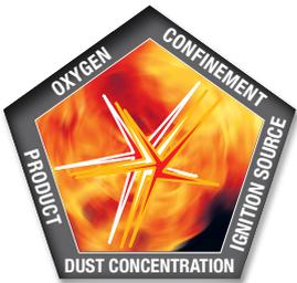
During the mixing or transport of products dust atmospheres can be created. Hot spots or smoldering fires can enter in mixers or containers. The products can also ignite itself by exothermic processes or sparks. The risk of a dust explosion is given with appropriate air atmosphere ( $O_2$ ).
